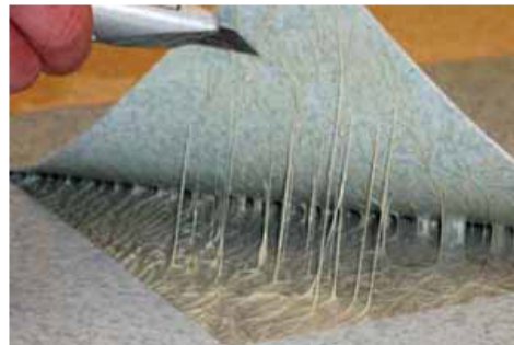
Figure 2 – Re-emulsified vinyl composition tile adhesive.
